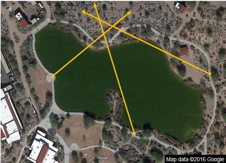
In this case google earth is used, to plot bearing lines, but a local area map of suitable size will work as well.
