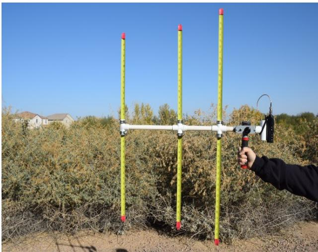
Tape measure yagi antenna
