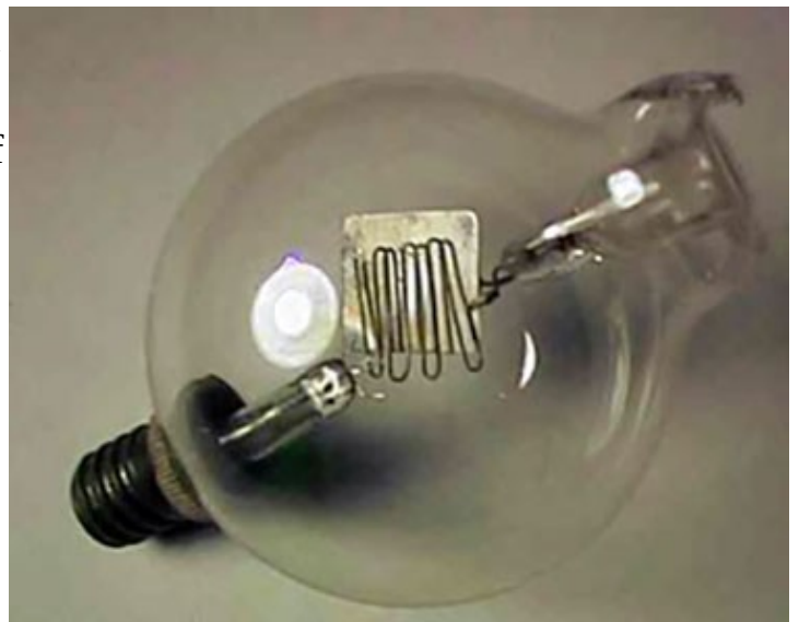
FIGURE 1. A photo of de Forest's Audion, the first vacuum tube triode.
